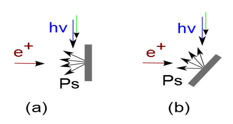
Figure 1: Time-bunched positron pulses incident on a porous silica target. (a) perpendicular arrangement for vacuum positronium studies. (b) Angled arrangement for inner-sample positronium studies.
